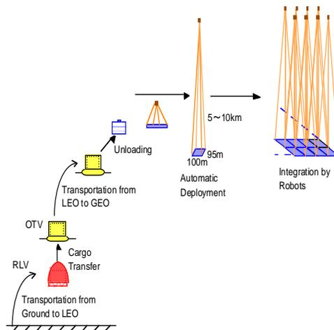
Fig.1 SSPS typical construction scenario.
