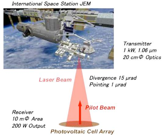
Fig.8 Laser power transmission experiment on the International Space Station.
