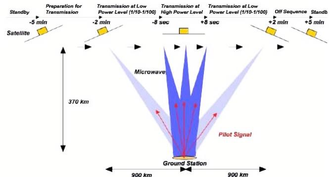
Fig.7 Experiment sequence of microwave transmission experiment.
