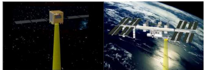
Fig.6 Microwave power transmission experiment in space on a small satellite (left) and on the International Space Station (right).
