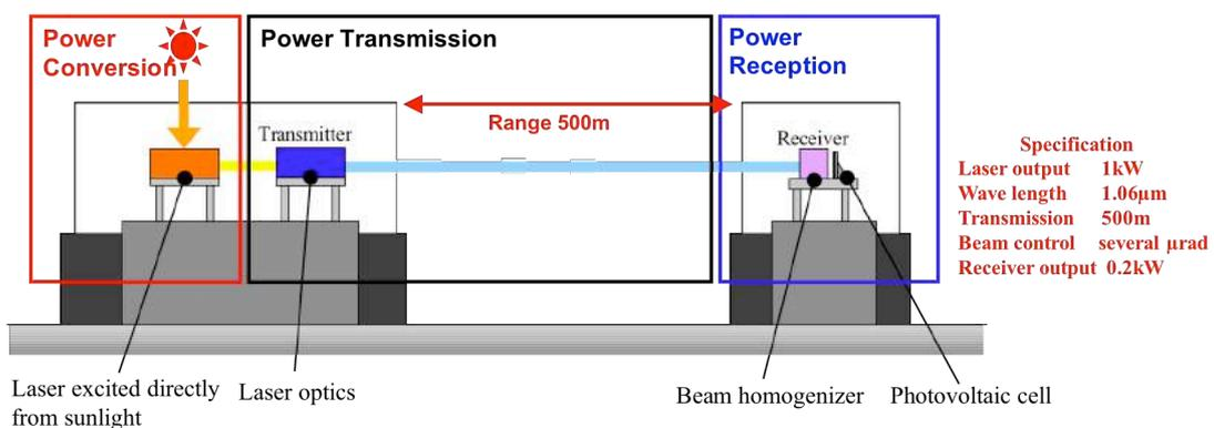
Fig.8 Laser transmission experiment on the ground.
