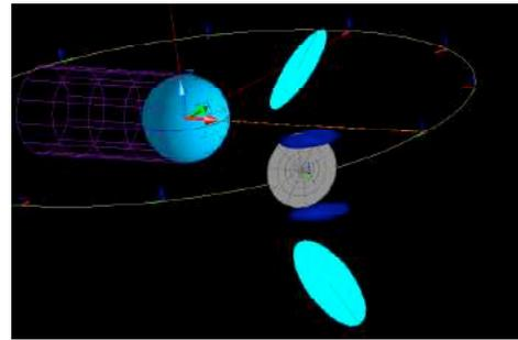
Fig.4 Formation flight model of reflective mirrors and power generation/transmission complex (JAXA).
