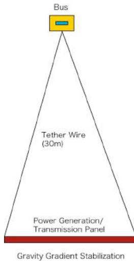
Fig.9 Configuration of the demonstration experiment using the small satellite.
