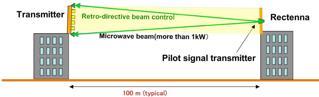
Fig.7 Microwave transmission experiment on the ground.
