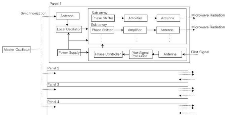
Fig.7 Microwave power transmission system for the ground experiment.
