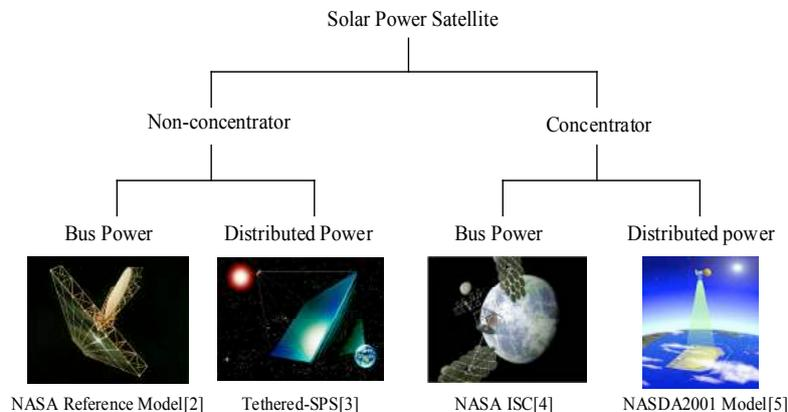
Fig. 1 Classification of microwave-type SSPS models and typical examples.
