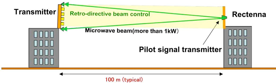
Fig.8 Configuration of the demonstration experiment on the ground.
