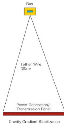
Fig.9 Configuration of the demonstration experiment using a small satellite.
