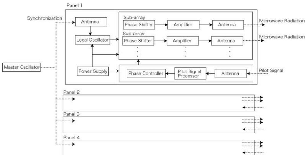
Fig.4 Block diagram of transmitting system.
