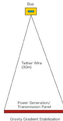
Fig.6 Configuration of the demonstration experiment in space.
