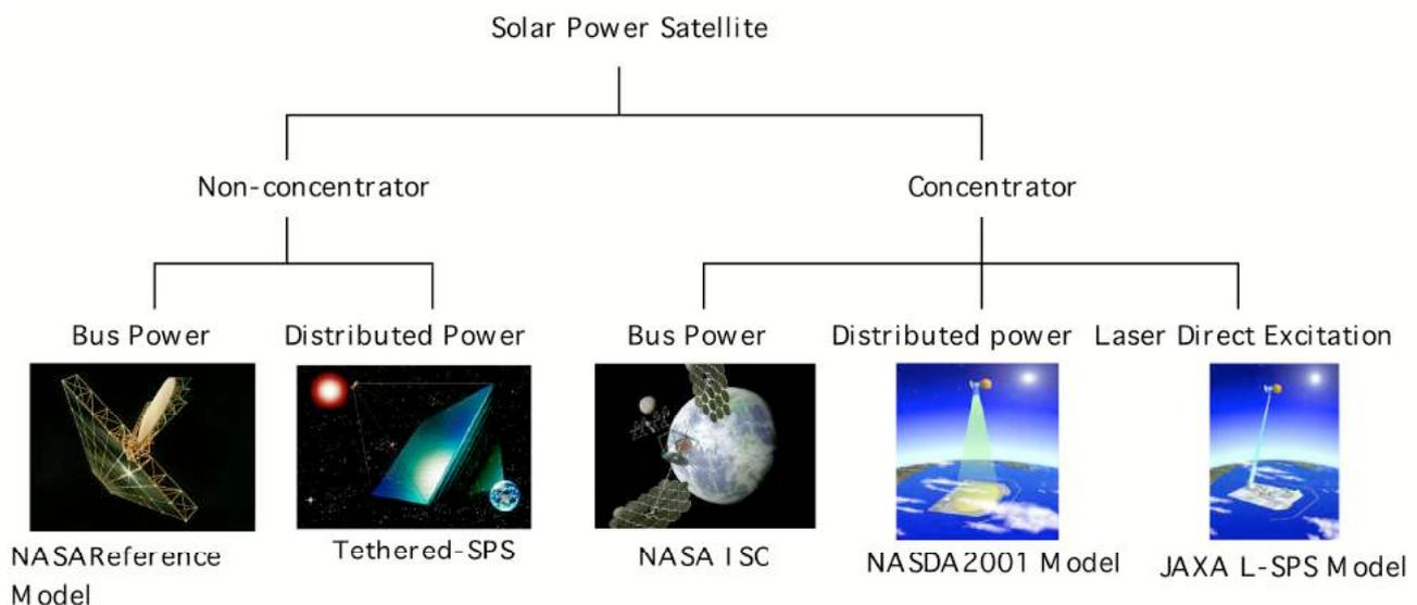
Fig.1 Classification of SSPS and typical examples of system configuration.
