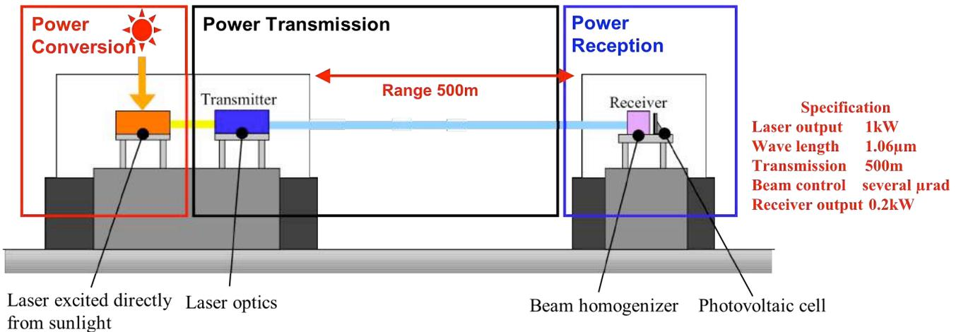
Fig.4 Basic concept of laser transmission experiment on ground.
