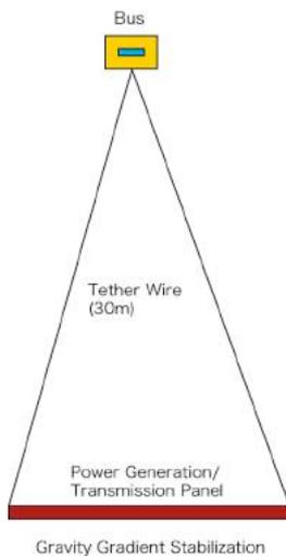
Fig.6 Configuration of the demonstration experiment (option A).
