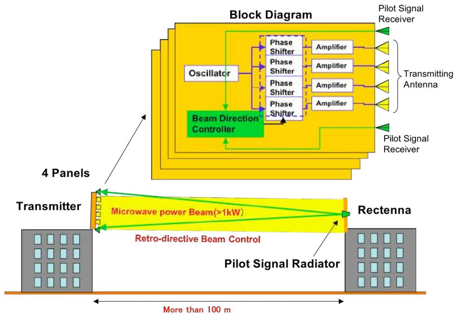
Fig.3 Basic concept of microwave transmission experiment on ground.
