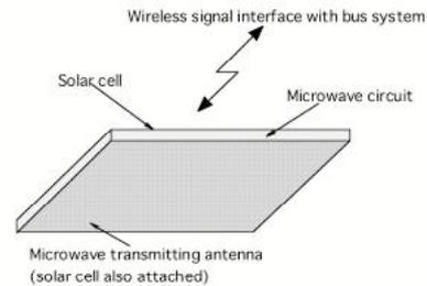
Fig.4 Configuration of Power generation/transmission module.
