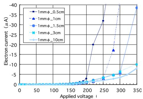
Fig.9 Dependence of current-voltage characteristics on electrode spacing (0.5cm-10cm). The size of the electrode is 1mm diameter. Enhancement in electron current is observed when the spacing of the electrode is equal to or less than 1.5 cm.
