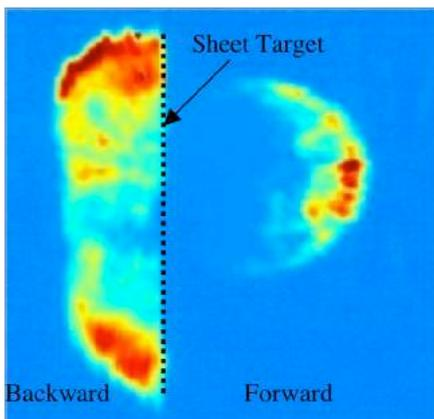
Fig.8 Propagation of impact plasma (right: forward propagation in spherical shape, left: propagation in rear side along the sheet target).
