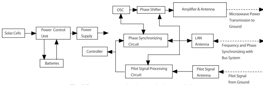
Fig.5 Power generation/transmission module.
