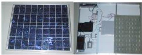
Fig.6 Laboratory test model of the power generation/transmission module. left: solar array. right: microwave circuits and antenna.
