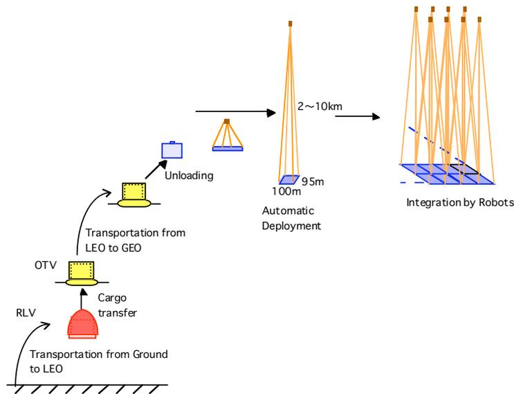
Fig.3 Transportation and construction scenario of Tethered-SPS.
