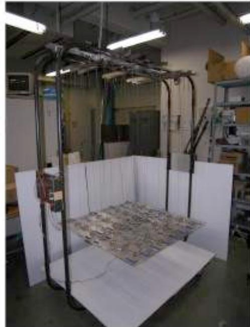
Fig.6 Demonstration of deployment of 4x8 miniature panels using SMA coils.
