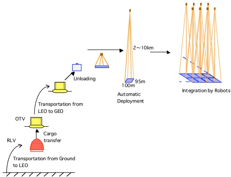
Fig.6 Construction scenario of Tethered-SPS.
