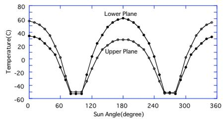
Fig.5 Temperature variation of the two panels in a day.
