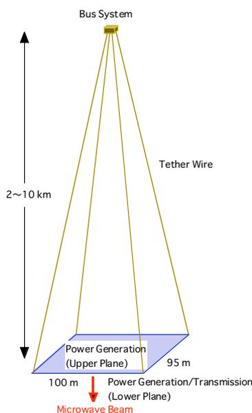
Fig.1 A unit of Tethered-SPS.
