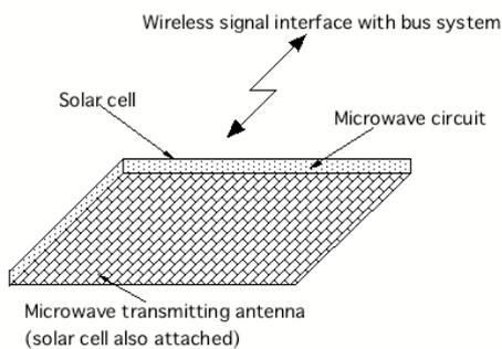
Fig.4 Concept of power generation/transmission module.
