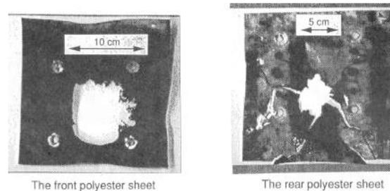
Fig 5 Typical examples of the hyper-velocity impact damage of a panel structure similar to the thin-film solar cell. The damage extended almost 10 times larger than the projectile scale (10 mm).
