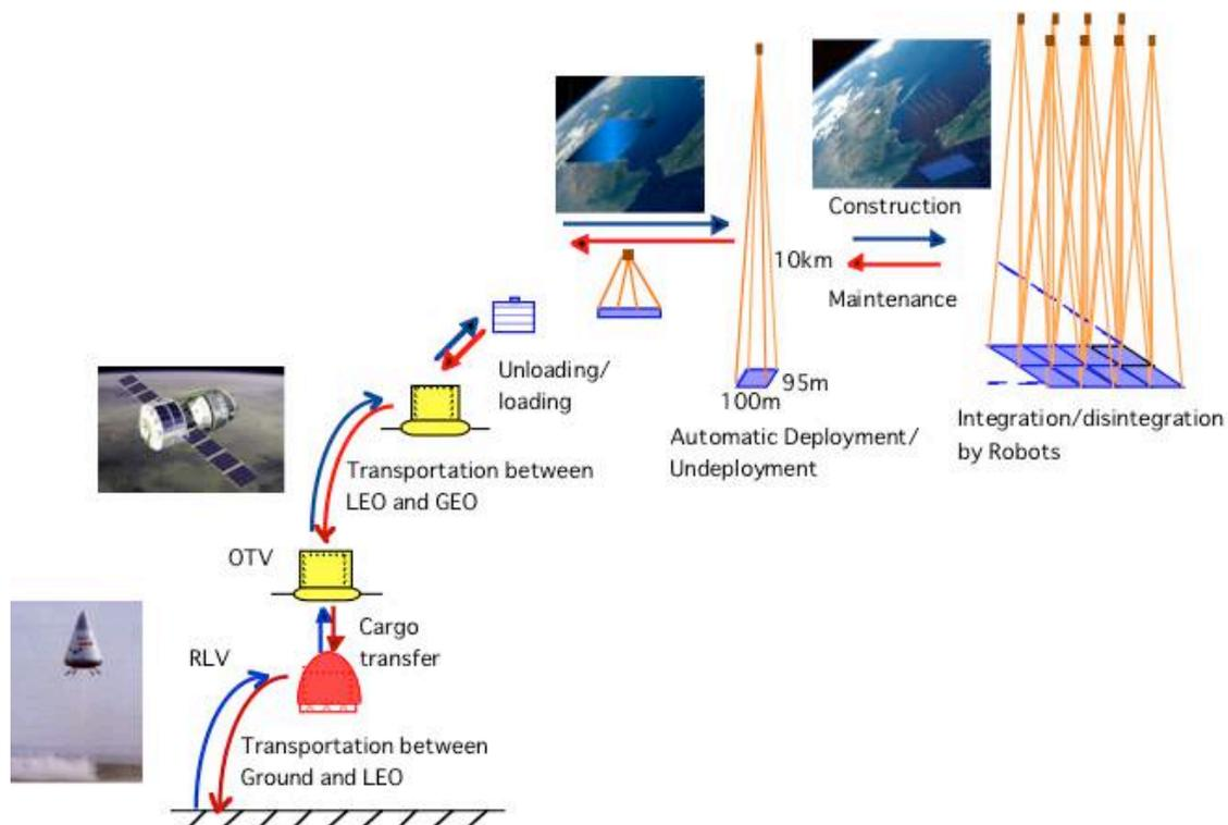
Fig. 6 Construction (blue) and maintenance (red) scenario.
