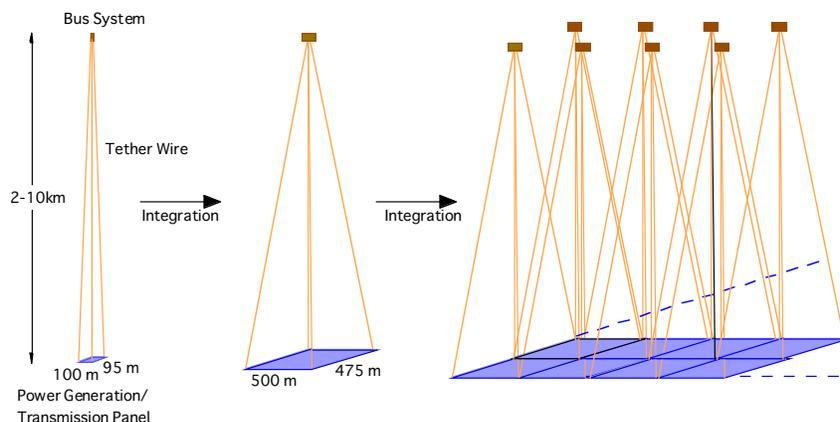
Fig.3 Unit of the Tethered-SPS and its integration process to a large-scale SPS.
