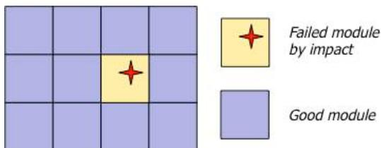
Fig 4 Modules are electrically isolated to each other so as that a failure in a module does not propagate to the other modules.
