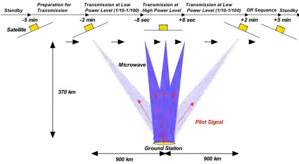
Fig.8 Experiment sequence in case of Mode A. The full power at 3.8 kW is transmitted to the ground for 16 sec guided by the pilot signal when the satellite is flying over the ground station.
