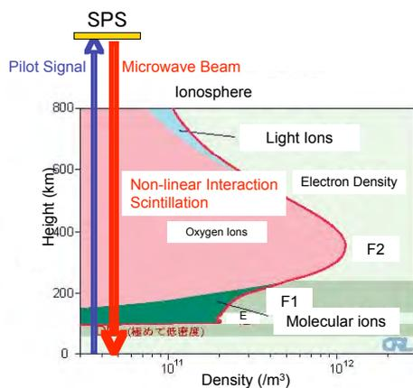
Fig.5 Study of interaction of microwave and ionospheric plasma.
