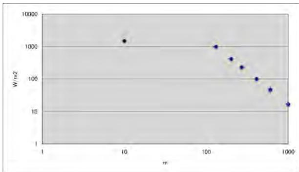
Fig.10 Microwave power intensity vs the distance from the transmitter in case of JEM experiment.
