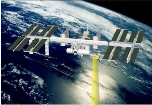
Fig.9 Microwave power transmission experiment at 8.64 kW from the Space Station JEM.
