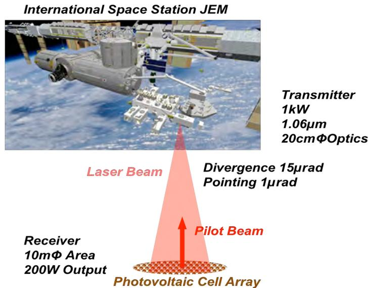
Fig.12 An example of laser power transmission experiment from the Space Station JEM.
