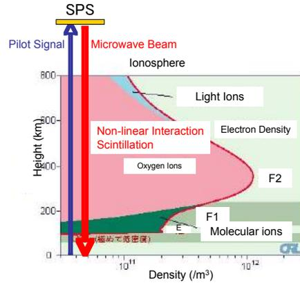
Fig.5 Possible interaction of the main beam and pilot signal with the ionospheric plasma.
