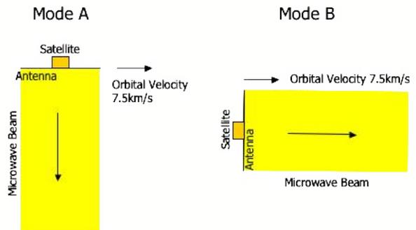
Fig.6 Two configurations of the demonstration experiment using a small satellite. The microwave beam is transmitted to the ground in mode A, while it is transmitted parallel to the orbiter velocity vector in mode B.
