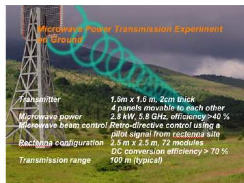
Fig.3 Microwave power transmission experiment on the ground.
