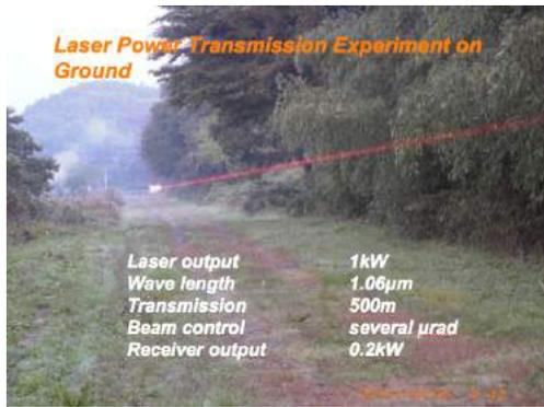
Fig.4 Laser power transmission experiment on ground.
