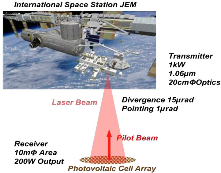
Fig.9 Laser power transmission experiment from the Space Station JEM.
