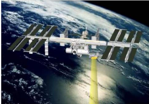
Fig.7 Microwave transmission experiment at 6.3 kW using the Space Station JEM.
