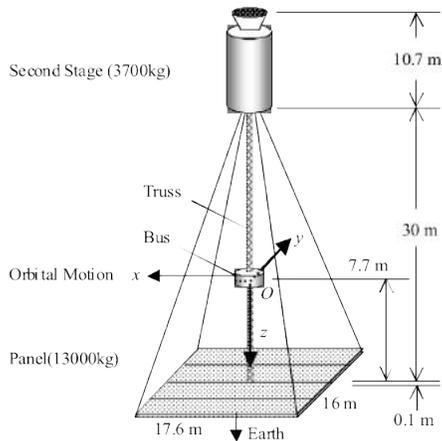
Fig.7 100kW class demonstration experiment in space.
