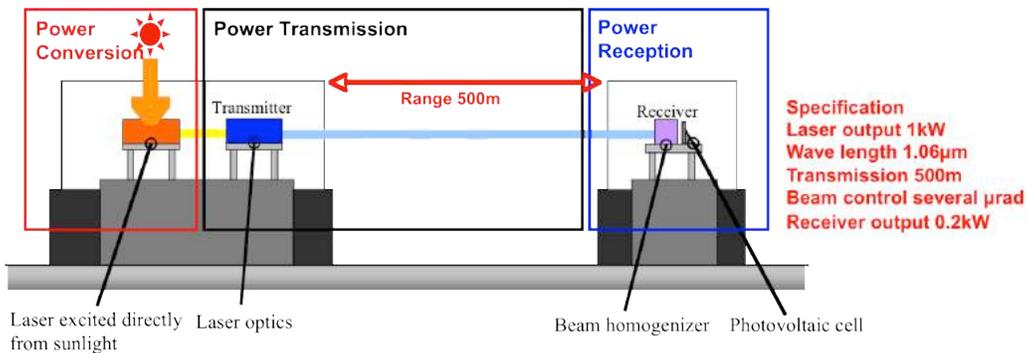
Fig.5 Laser power transmission experiment on the ground.
