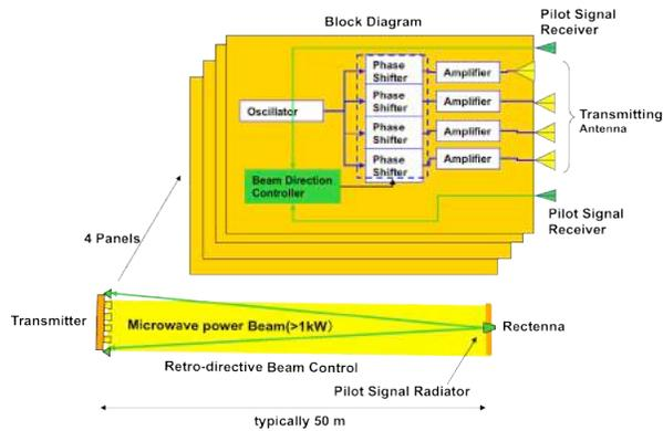
Fig.4 Microwave power transmission experiment on the ground
