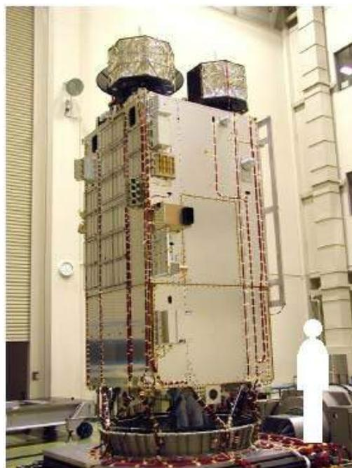
Fig.9 SELENE Mechanical Test Model
