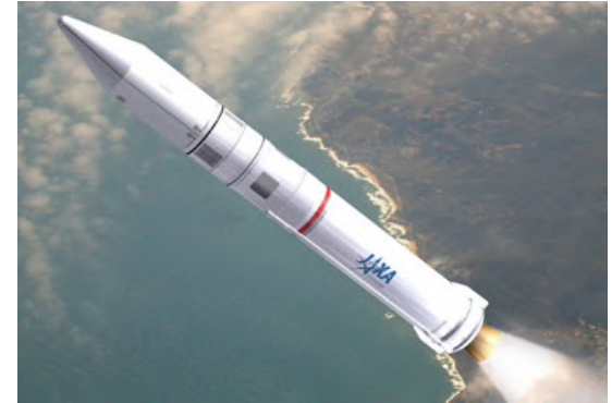
Epsilon Launch Vehicle for small satellite. Next-generation solid propellant rocket after the former M-V launch vehicle.
