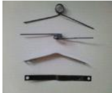
Actuator using shape memory alloy coils
